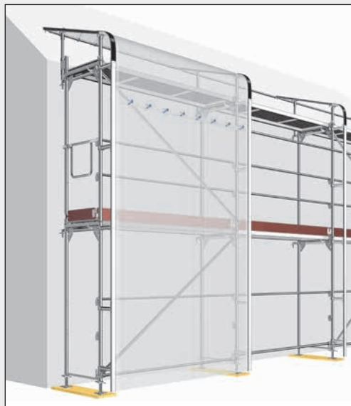
Keder tarpaulins in use on the scaffolding
