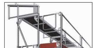
Top scaffolding guardrail, secure assembly thanks to lower bracket levels
